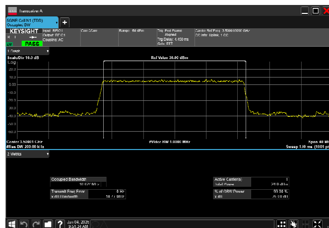
n77_1_20MHz_30kHz_3500MHz_DFT-s-OFDM QPSK_RB50@0 Occupied Bandwidth 26 dB Emission Bandwidth
