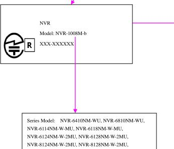
The Label's material is silk-screen, it cannot be easily erased. The size for the label is 60mm\*20mm The MIC Logo height is 3mm\*3mm. The Printing Color is White and Black.
