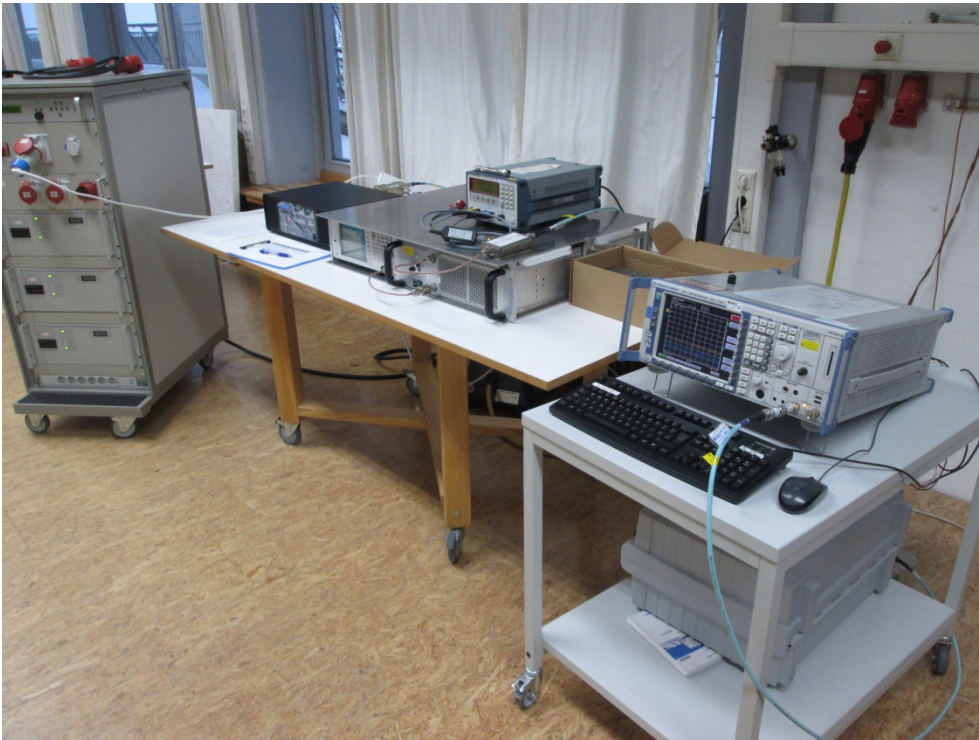
Photo A1-1: conducted spurious emissions measurement
