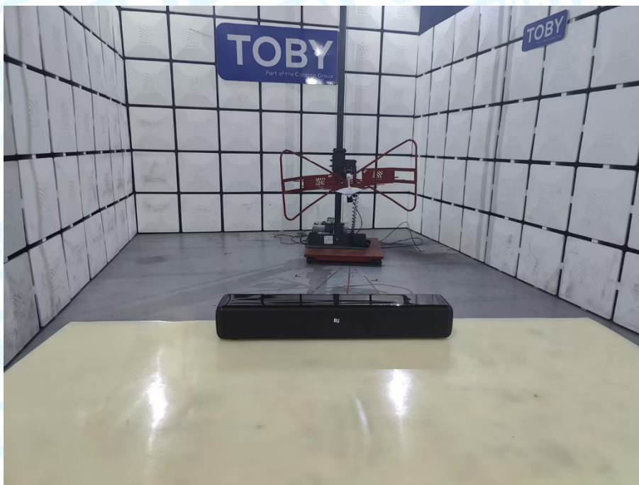
Photo of Setup for Radiated Emission (30MHz~1GHz)
