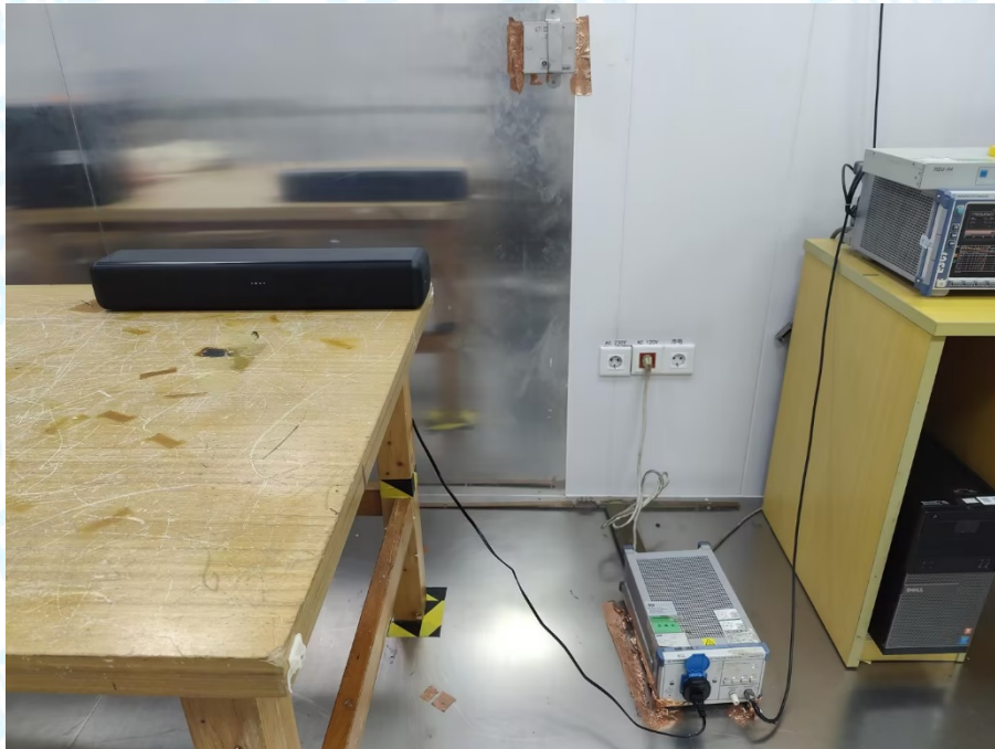
Photo of Setup for Radiated Emission (30MHz~1GHz)
