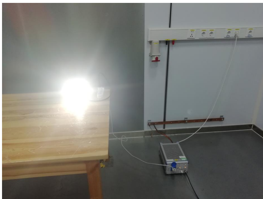
Fig. 4 Power line conducted emission setup photo
