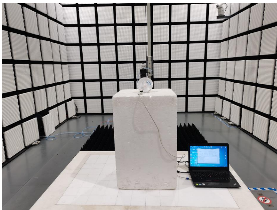
Fig. 3 Radiated emission setup photo(Above 1GHz)
