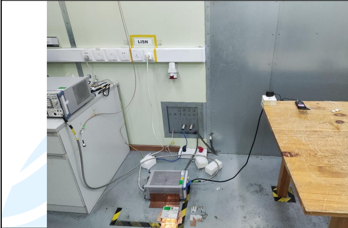
Conducted Emission Test Setup
