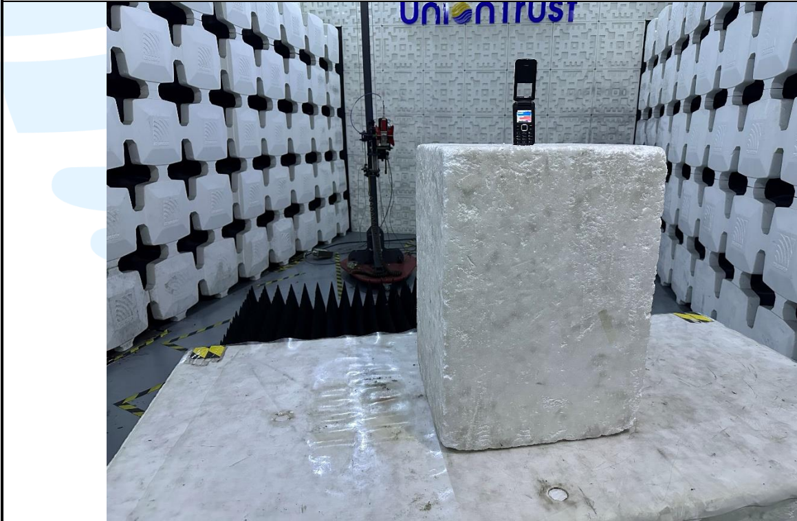
Radiated emission Test Setup (Above 1 GHz)
