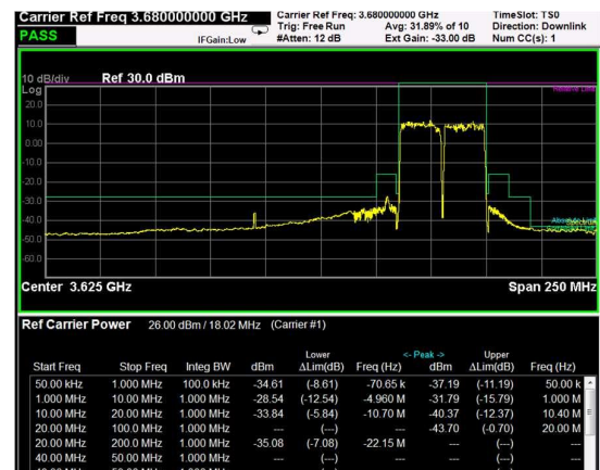
High Band Edge, 2 Carrier, Modulation: 256QAM, BW=20MHz
