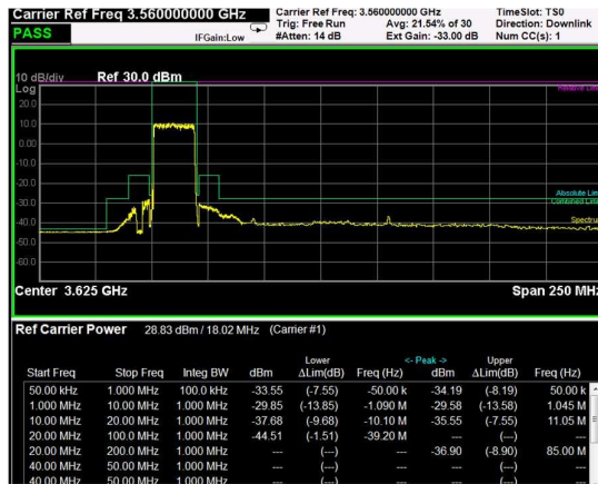
Low Band Edge, 1 Carrier, Modulation: 16QAM, BW=20MHz
