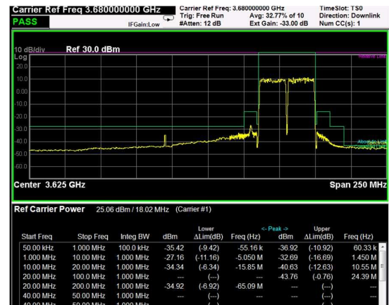
High Band Edge, 2 Carrier, Modulation: 64QAM, BW=20MHz
