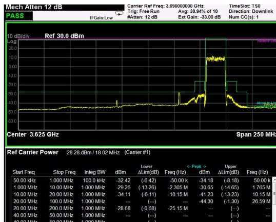
High Band Edge, 1 Carrier, Modulation: 64QAM, BW=20MHz
