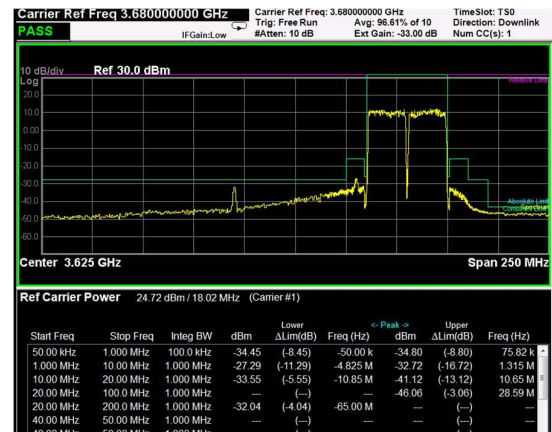
High Band Edge, 2 Carrier, Modulation: QPSK, BW=20MHz
