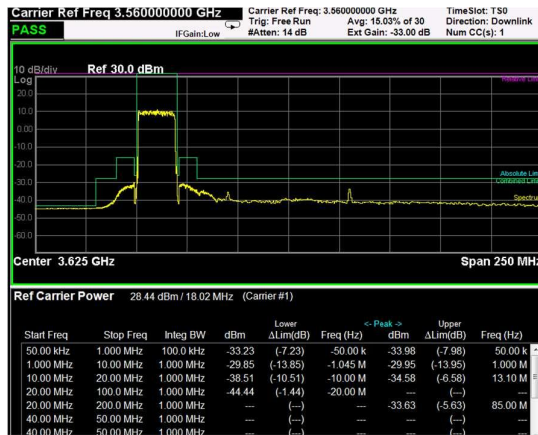
Low Band Edge, 1 Carrier, Modulation: 256QAM, BW=20MHz
