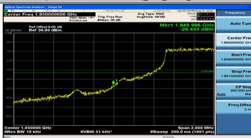
(Channel Bandwidth: 1.4 MHz)_LCH_QPSK_3RB#3
