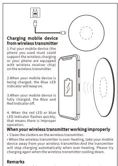
1.The wattage of the power adapter you used need more than 7.5W, We suggest you use the adapter with 5V/2A output.
