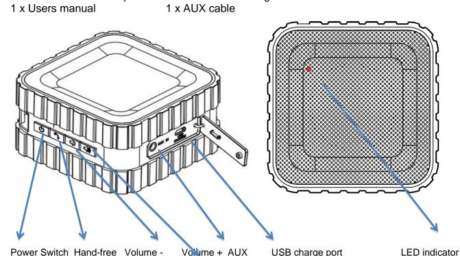
Power Switch Hand-free Volume - Volume + AUX USB charge port Charging the HR-686 (3.7V 800mAh rechargeable battery built-in)
