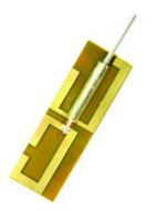
The Laird Connectivity Mini NanoBlade Flex antenna features a flexible printed circuit board that supports WLAN applications. The flexible board can be embedded in space-sensitive applications where a curved housing does not provide a flat surface for antenna mounting. The antennas are specifically designed to be embedded inside devices for aesthetically pleasing integration.
