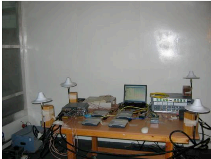
Photograph 1.14.1 Setup for conducted emission measurements
