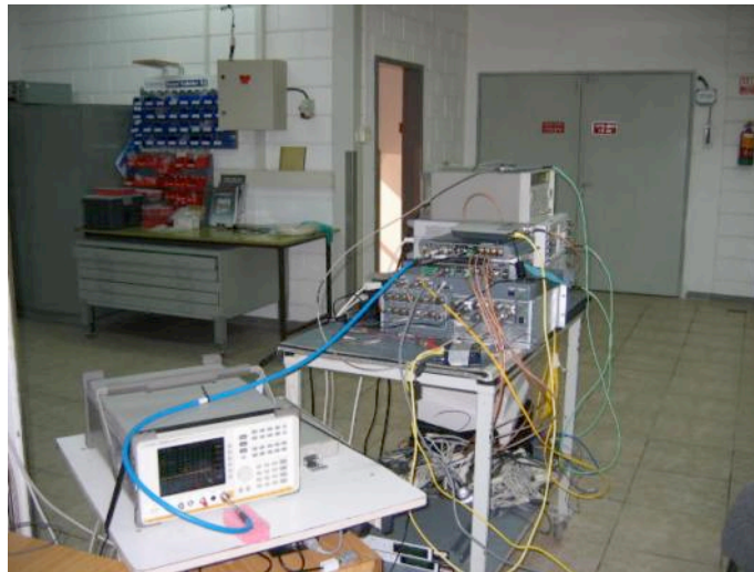
Photograph 1.11.1 Peak spectral power density test setup
