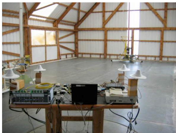
Photograph 1.10.3 Setup for spurious emission field strength measurements above 1000 MHz
