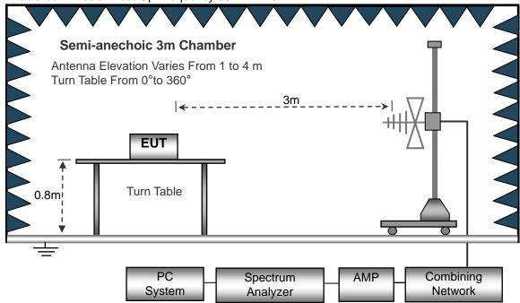
(C) Radiated Emission Test-Up Frequency Above 1GHz
