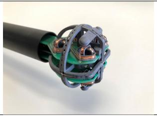
Test probe, without the casing
