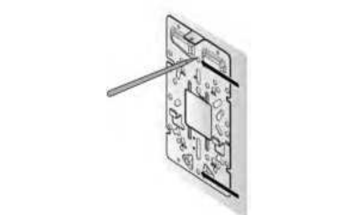
Figure 3 Wall installation holes
