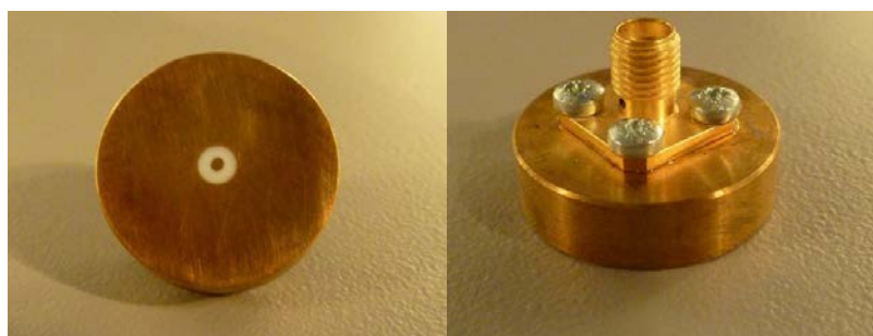
Figure 1 – MVG LIMESAR Dielectric Probe
