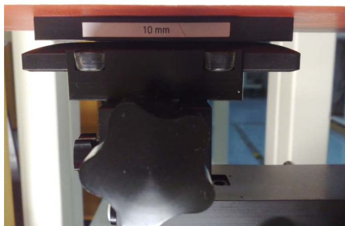
Photo of the device positioned for WR mode measurement –back facing phantom. The spacer was removed before the start of the measurements.
