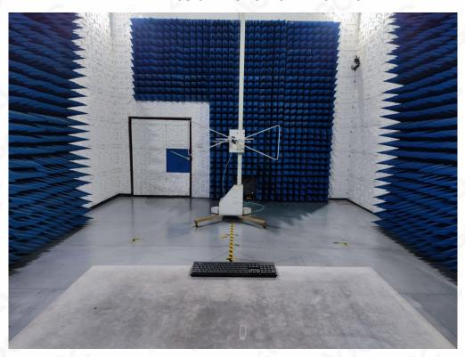
RADIATED EMISSION TEST SETUP ABOVE 1GHz
