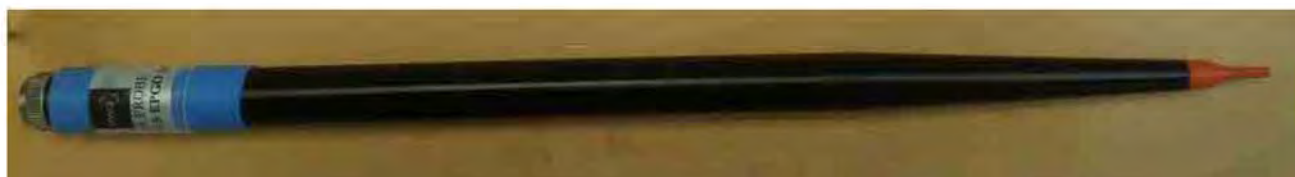
Figure 1 – MVG COMOSAR Dosimetric E field Dipole
