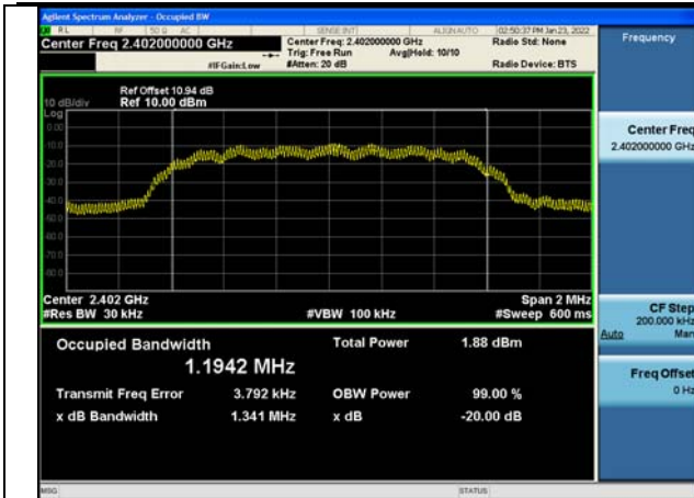
Test Mode: \pi/4 DQPSK(2DH5) MHz
