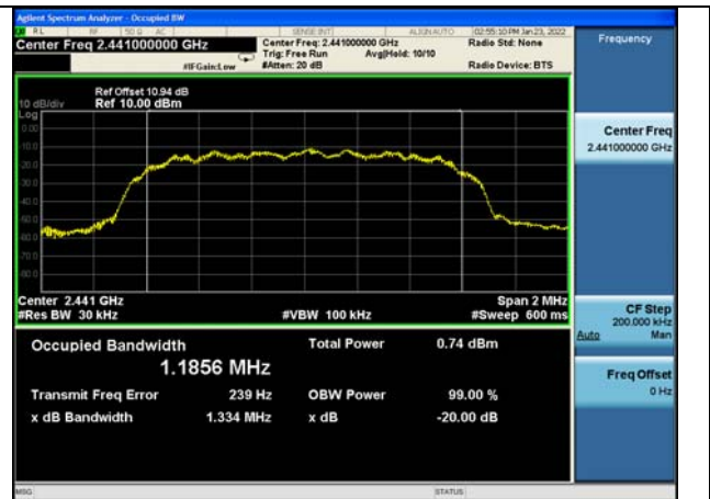
Test Mode: \pi/4 DQPSK(2DH5) MHz
