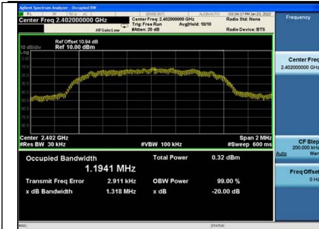
Test Mode:8DPSK(3DH5) MHz
