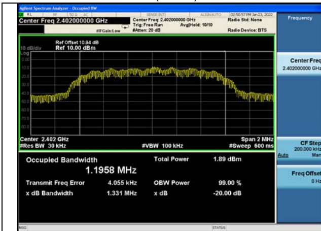
Test Mode: \pi/4 DQPSK(2DH5) MHz
