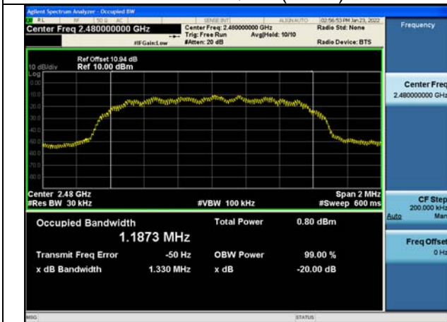
Test Mode: \pi/4 DQPSK(2DH5) MHz
