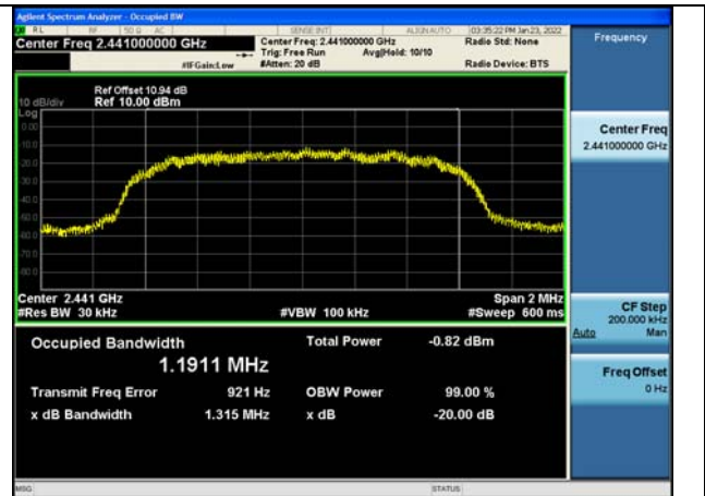
Test Mode: 8DPSK(3DH5) MHz
