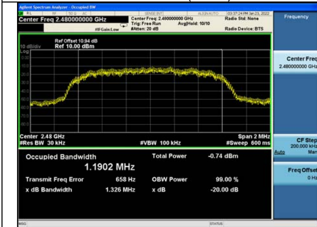
Test Mode:8DPSK(3DH5) MHz
