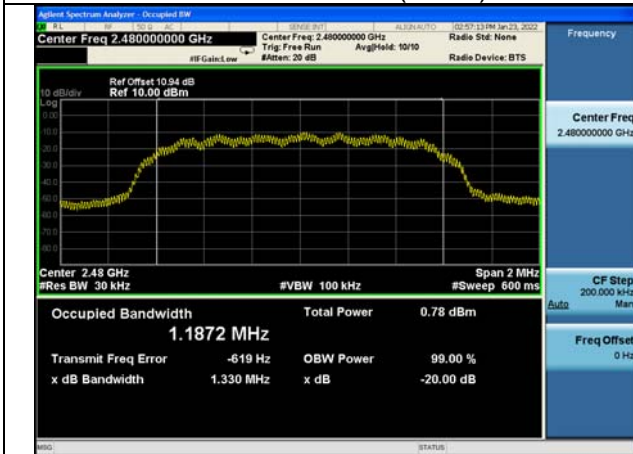
Test Mode: \pi/4 DQPSK(2DH5) MHz
