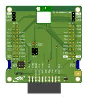
**Integrated PCB Trace Antenna for BDE-BW33PA Module Series**
