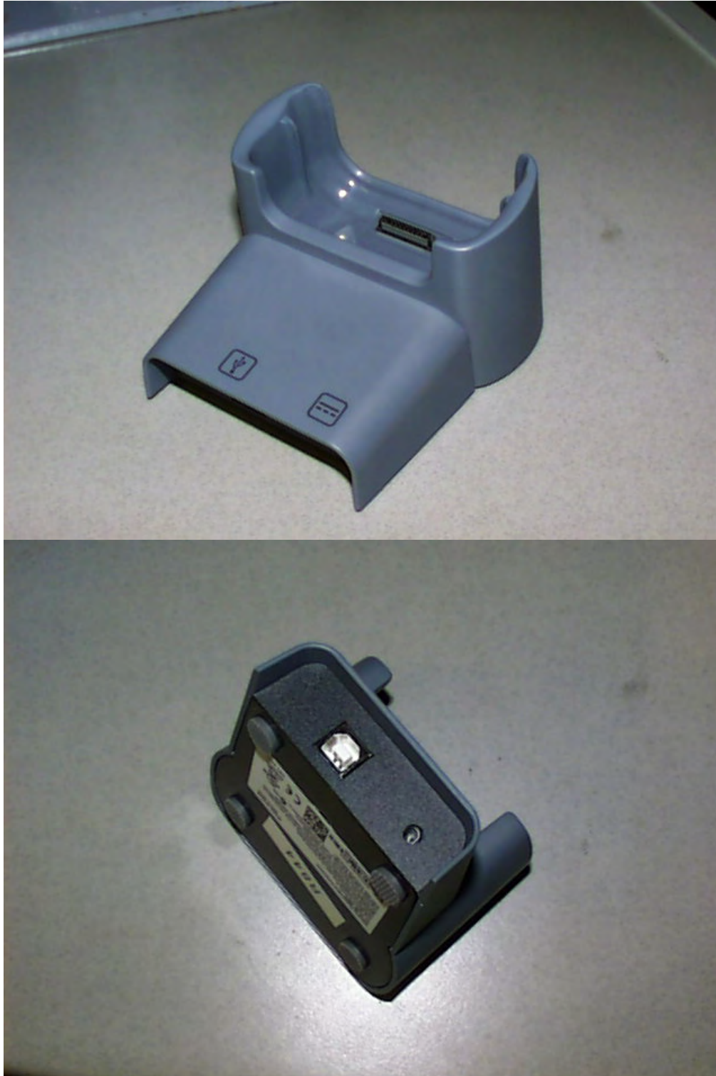
CN2B Charging dock rear view and connectors
