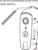
2. Unscrew the security screw and remove the cover of the doorbell. Place against the surface you would like it to be mounted. Mark each screw hole with a pencil (as displayed
