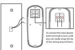
It does not matter which wire attaches to which terminal. If the original wiring is not long enough, use the supplied extra
