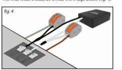
4. Position the power bypass kit within your doorbell, away from any moving parts. Use the supplied stickers on the back of the power bypass kit to keep it in place and slide the cover back onto your doorbell.
