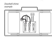
1. Remove the cover from your doorbell. Loosen and undo the terminal screw labelled "Front" (fig.1).
