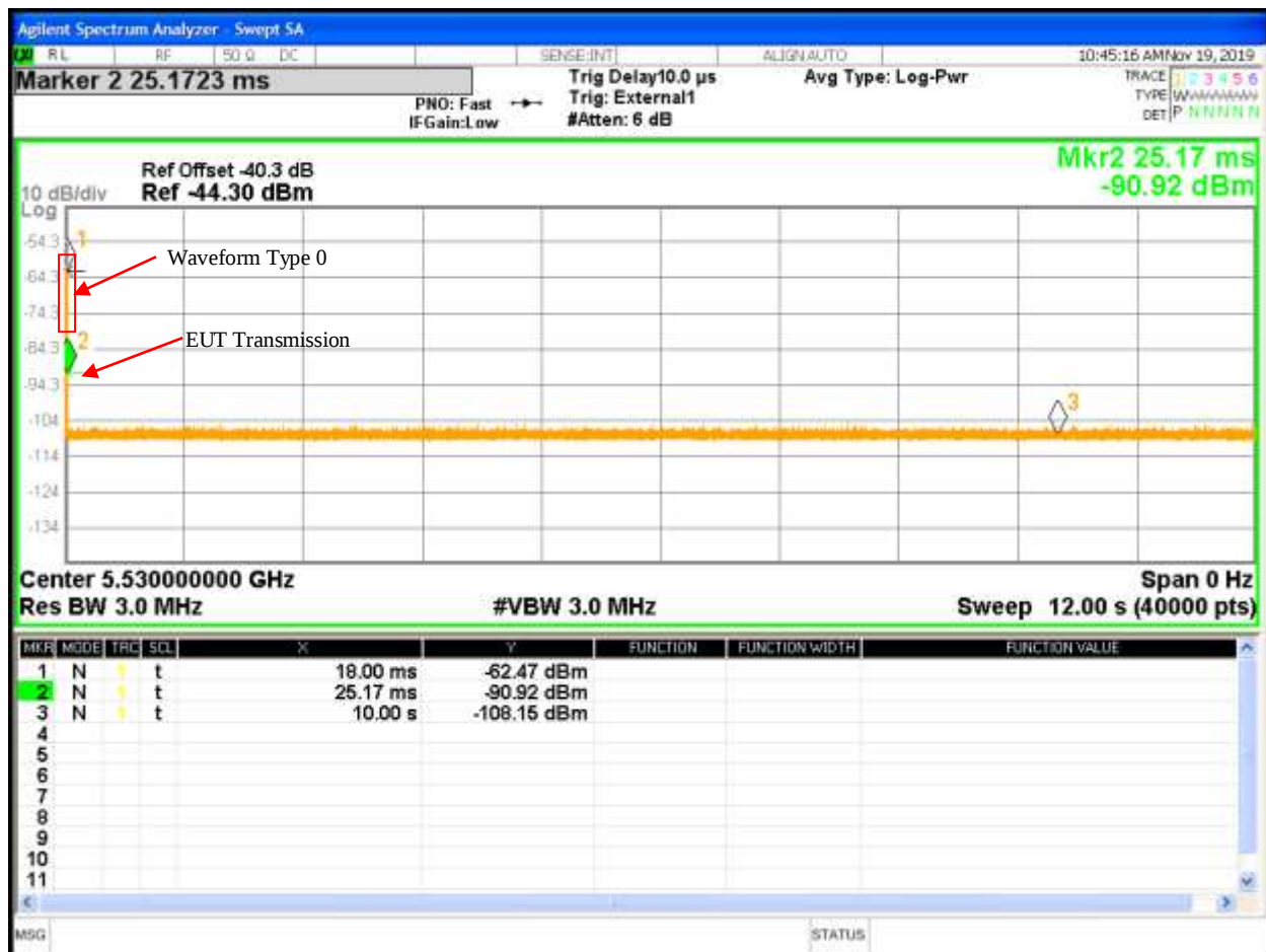
Figure 18: Channel Move Time and Channel Closing Transmission Time using Pulse Radar Waveform 0 in Master Mode 11AC VHT80, 80 MHz Bandwidth
