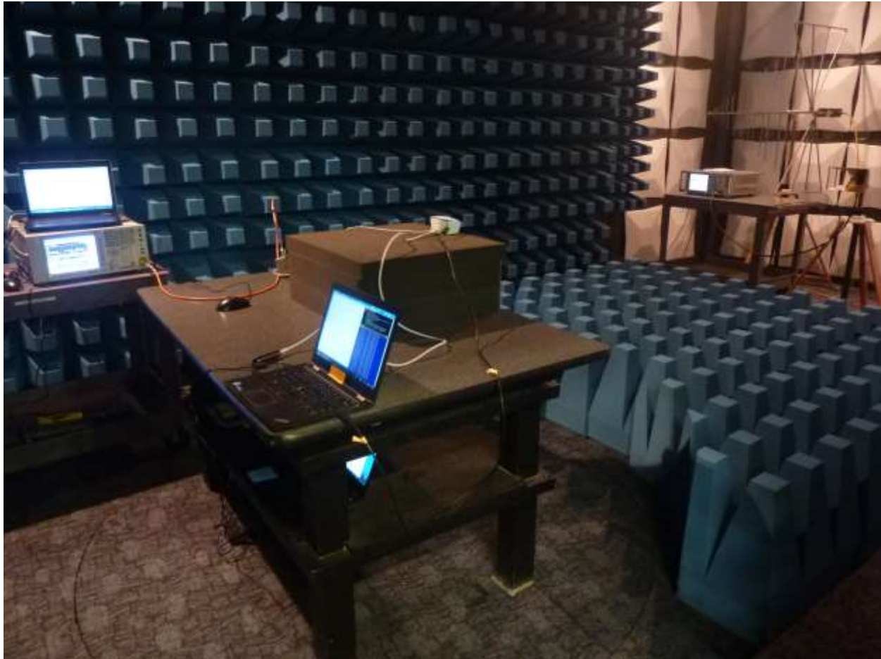
Figure 22: DFS Test Setup Photo for Master – Radiated Method – View 2
