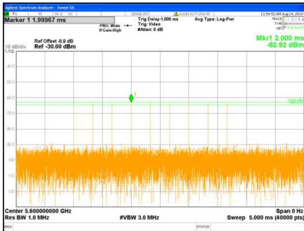
Figure 8: Radar Type 6 DFS Detection Threshold Level at 5600 MHz (9 Pulses in Burst)
