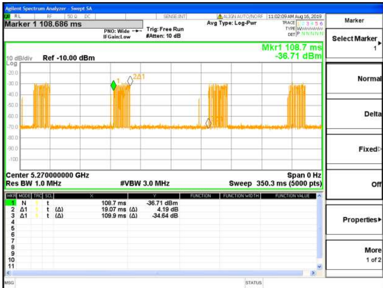
Figure 10: EUT Channel Loading at 5270 MHz. (40 MHz bandwidth)
