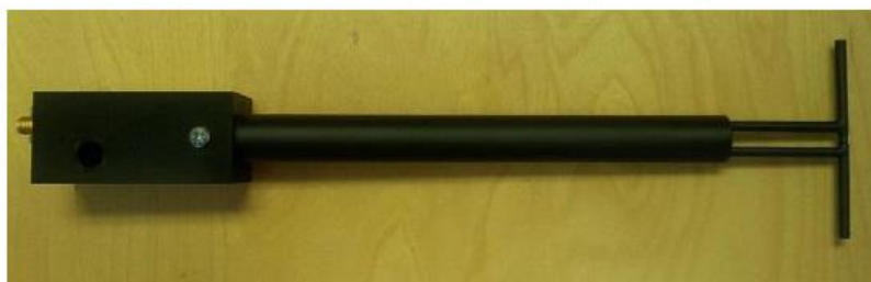
Figure 1 – MVG COMOSAR Validation Dipole
