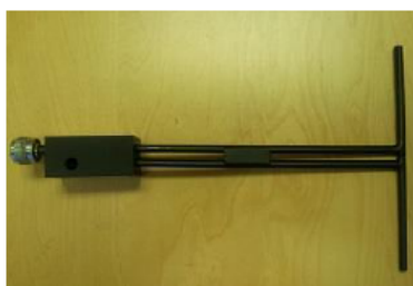
Figure 1 – MVG COMOSAR Validation Dipole
