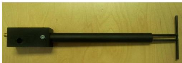
Figure 1 – MVG COMOSAR Validation Dipole
