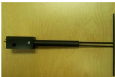
Figure 1 – MVG COMOSAR Validation Dipole
