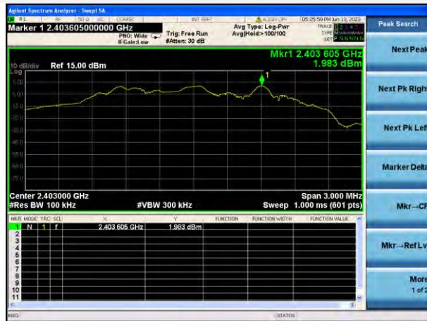
GFSK LOW CHANNEL, CARRIER LEVEL
