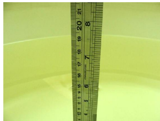
Fig 7.2 Photo of Liquid Height for Body SAR
