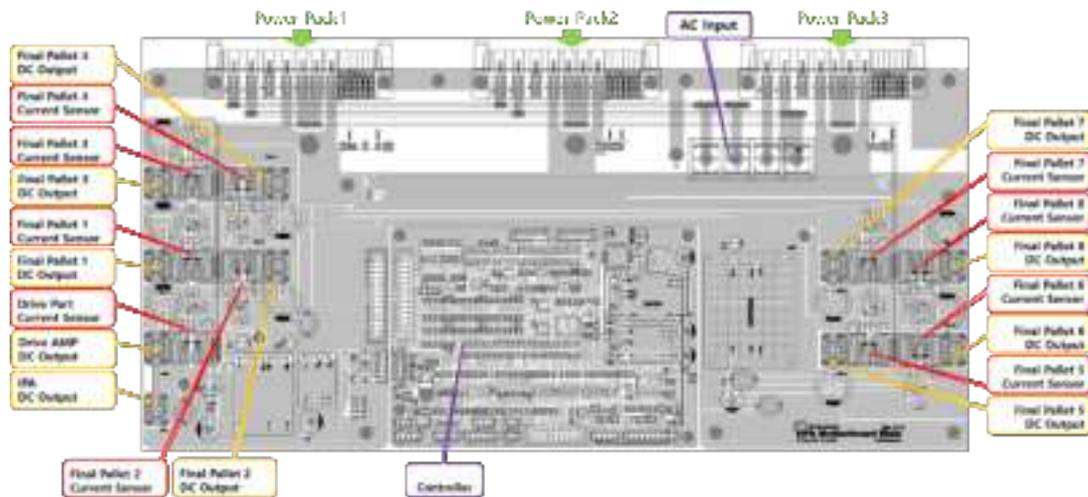
Motherboard includes Interface function, Current Sensing, and DC-DC Converter function.
