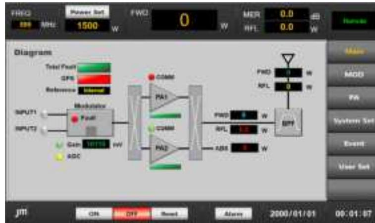
Displays information of each Transmitter's Path on one screen.
