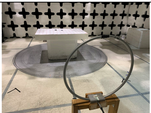
Radiated Emission Test below 30MHz Rear View
