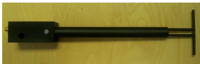
Figure 1 – MVG COMOSAR Validation Dipole
