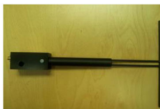
Figure 1 – MVG COMOSAR Validation Dipole
