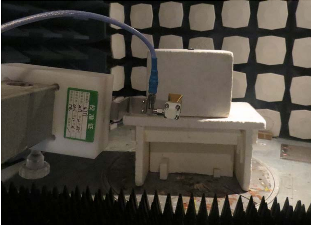
Picture 1: Radiated Spurious Emissions Test setup
