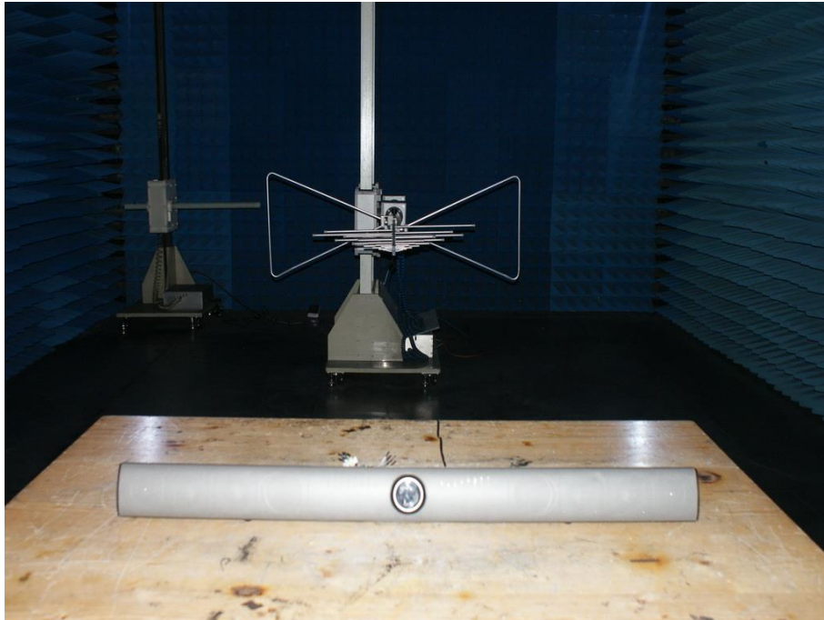
Photograph 5: Set-up for Radiated Spurious Emission, 30MHz - 1GHz
