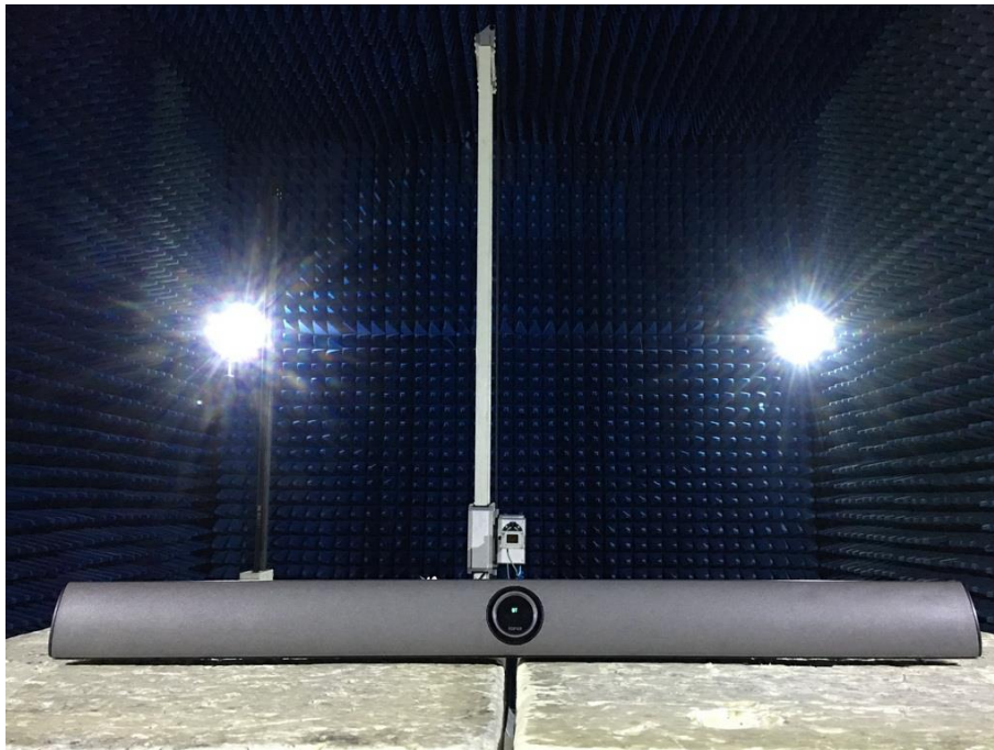
Photograph 7: Set-up for Radiated Spurious Emission, 18GHz - 26.5GHz
