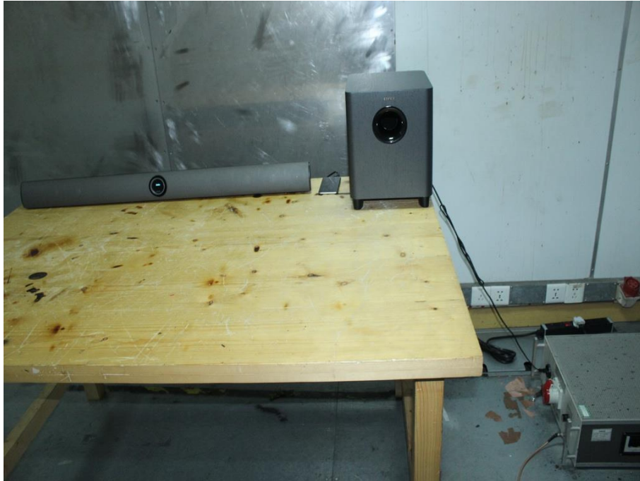
Photograph 1: Set-up for Conducted Emission on AC Mains
