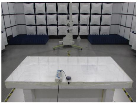
RADIATED EMISSION TEST (Frequency above 1GHz)
