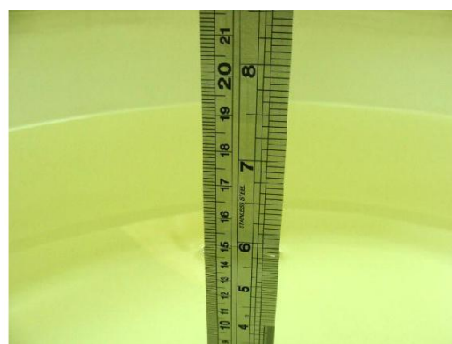
Fig 7.2 Photo of Liquid Height for Body SAR
