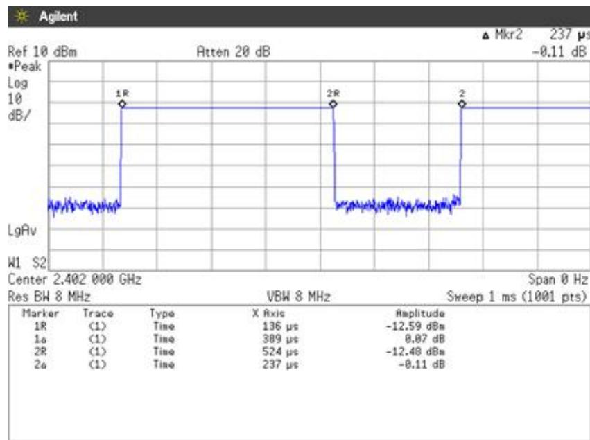
$$\text{Duty Cycle} = \text{Ton} / (\text{Ton} + \text{Toff}) = 389[\mu\text{s}] / (389[\mu\text{s}] + 237[\mu\text{s}]) = 62.14[\%]$$
