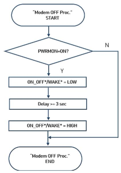
Figure 7: Modem OFF Process flow chart
