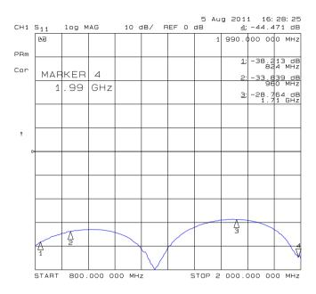
Figure 13: Return Loss plot of line under test
