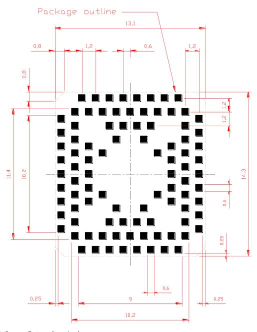
Figure 20: Copper Pattern (top view)
