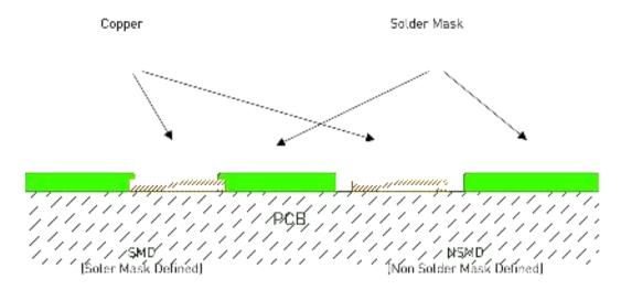
Figure 26: PCB solder pad recommendations
