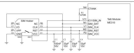
Figure 10: SIM Holder schematic
