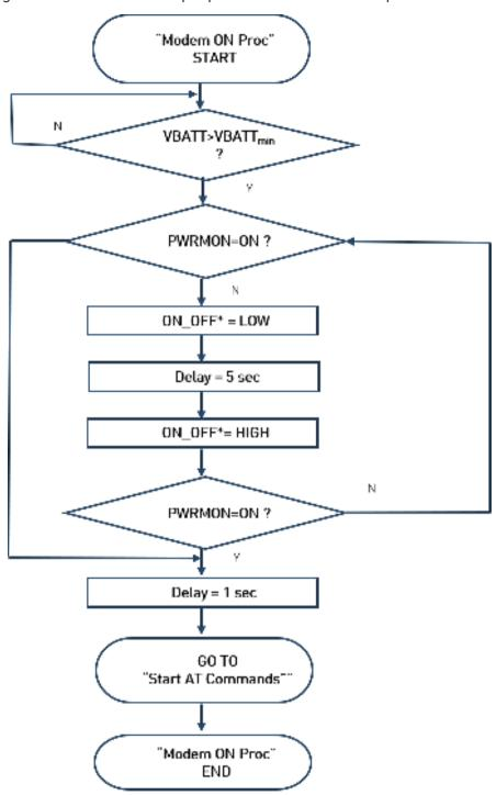
Figure 6: Modem On Process flow chart
