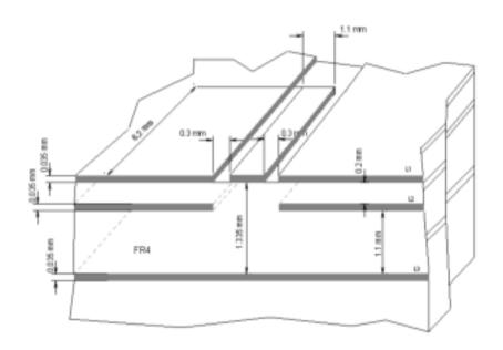
Figure 12: Line geometry
