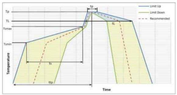
Figure 27: Recommended Solder reflow profile
