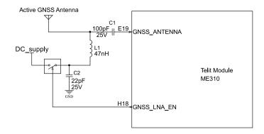
Figure 17: Antenna bias circuitry example
