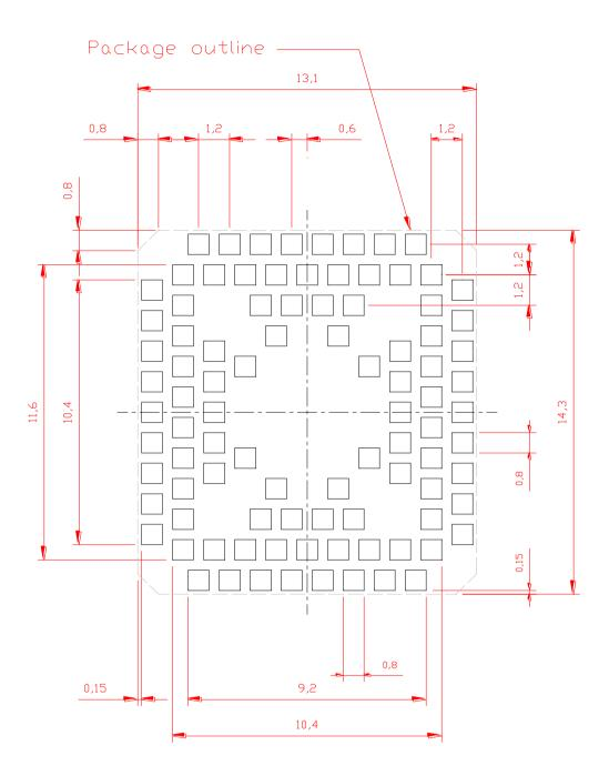
Figure 21: Solder resist pattern (top view)
