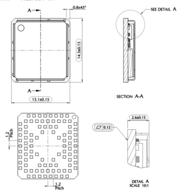
Figure 18: Mechanical Drawing of ME310G1-W1
