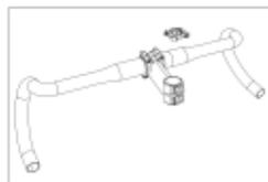
Step 1: Place the mount on the handlebar.
