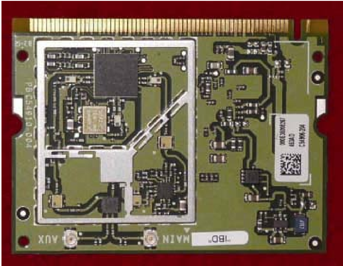
Front with Shielding Removed
