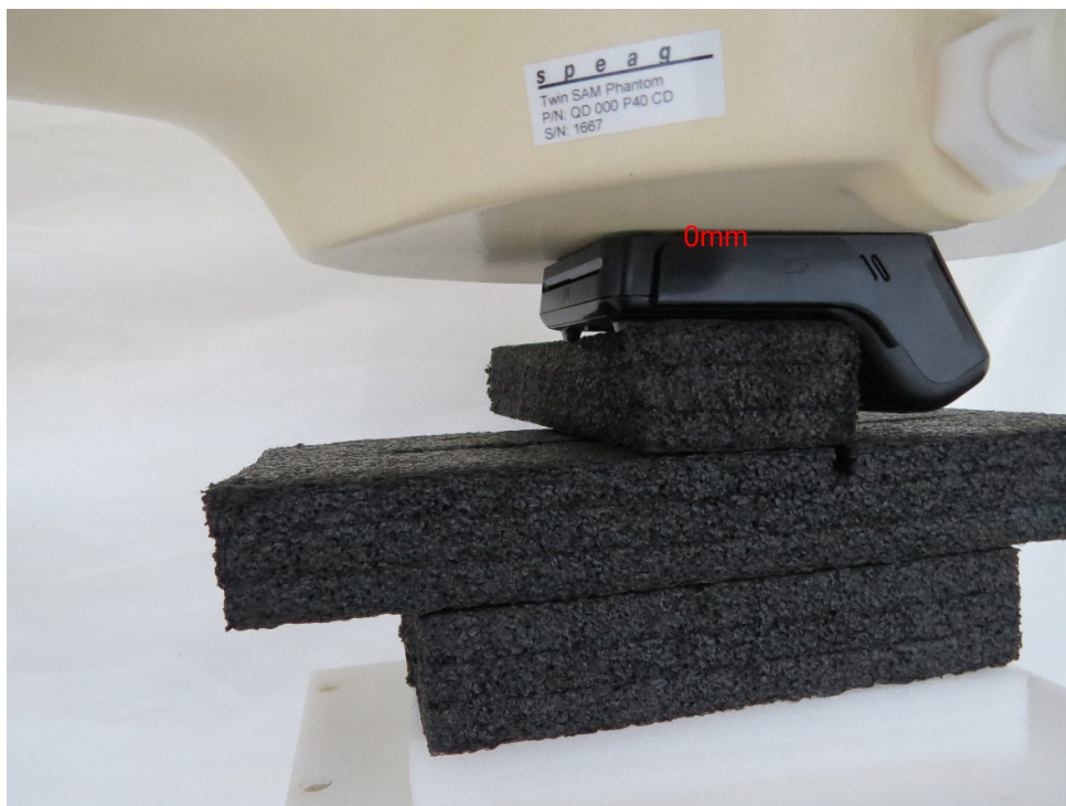
Picture 12: Front Side, the distance from EUT to the bottom of the Phantom is 0mm
