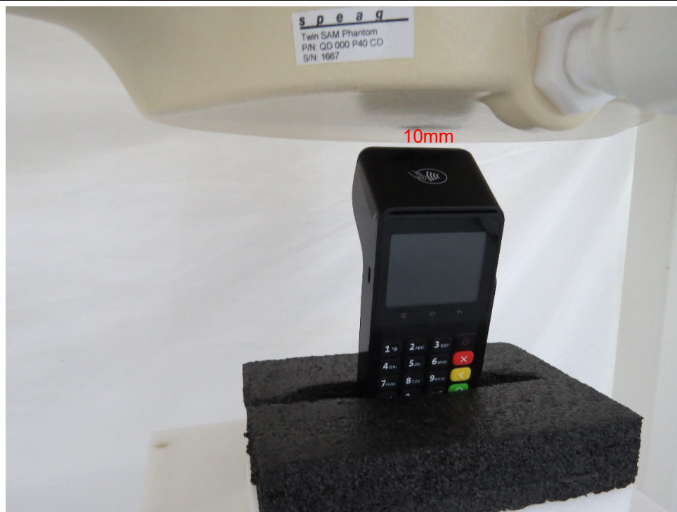
Picture 7: Top Edge, the distance from EUT to the bottom of the Phantom is 10mm
