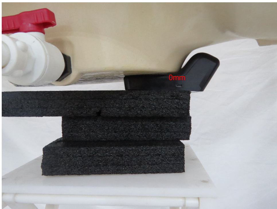
Picture 11: Back Side3, the distance from EUT to the bottom of the Phantom is 0mm
