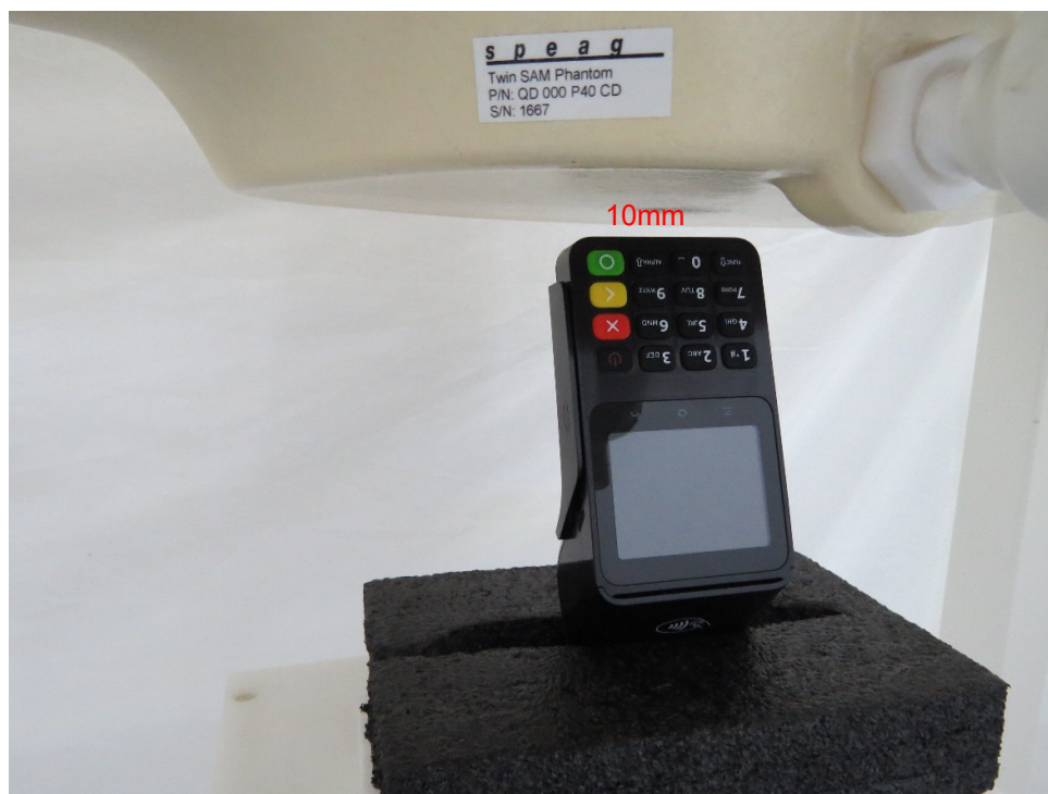
Picture 8: Bottom Edge, the distance from EUT to the bottom of the Phantom is 10mm
