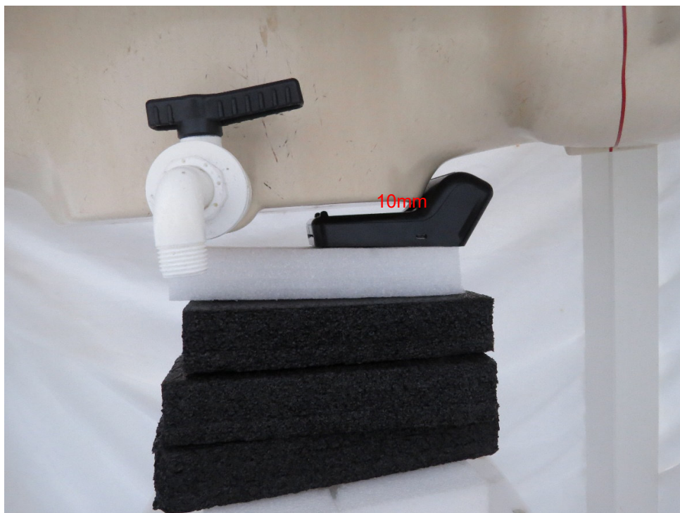
Picture 3: Back Side3, the distance from EUT to the bottom of the Phantom is 10mm
