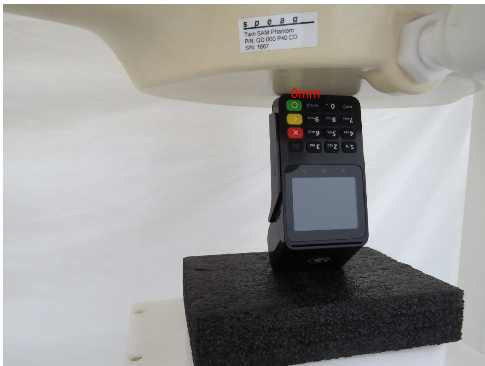
Picture 16: Bottom Edge, the distance from EUT to the bottom of the Phantom is 0mm
