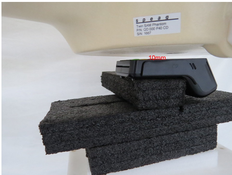
Picture 4: Front Side, the distance from EUT to the bottom of the Phantom is 10mm
