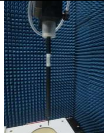
Fig.8.2 Photo of E-Field Probe
