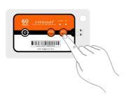
Long press "Start/Stop" button till red & blue LED indicators flash, the device is ready. Start delay is 15 min. (In this stage blue led will flash every 10 sec.), after delay time, the LED stop and the device start to record the temperature data. (Using default thresholds 0~30 °C ). Usage method is same as traditional USB logger.
