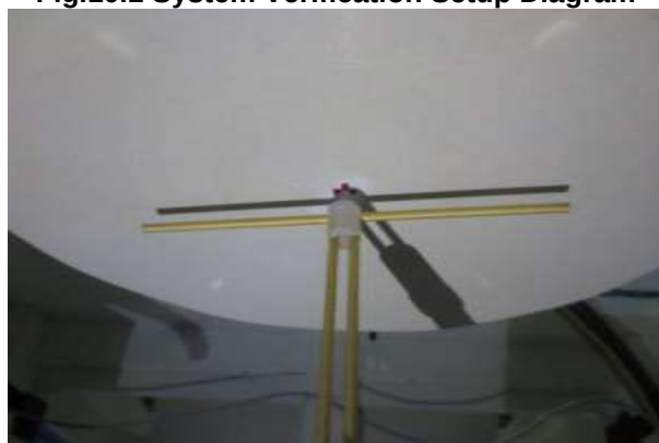
Fig.10.2 Photo of Dipole setup
