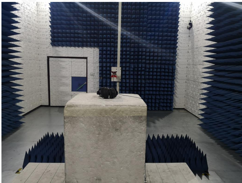
RADIATED EMISSION TEST SETUP ABOVE 1GHZ
