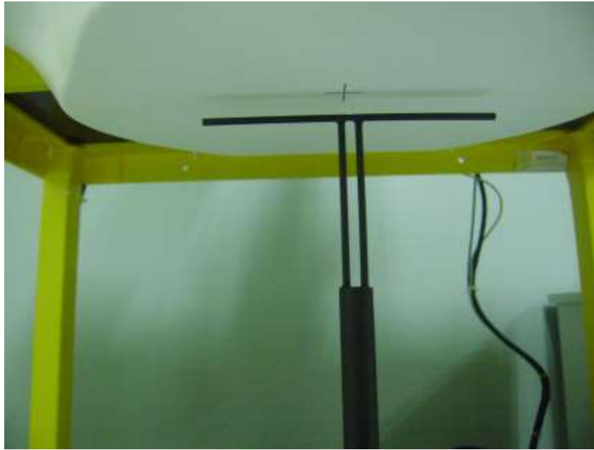
Setup Photo of Dipole Antenna
