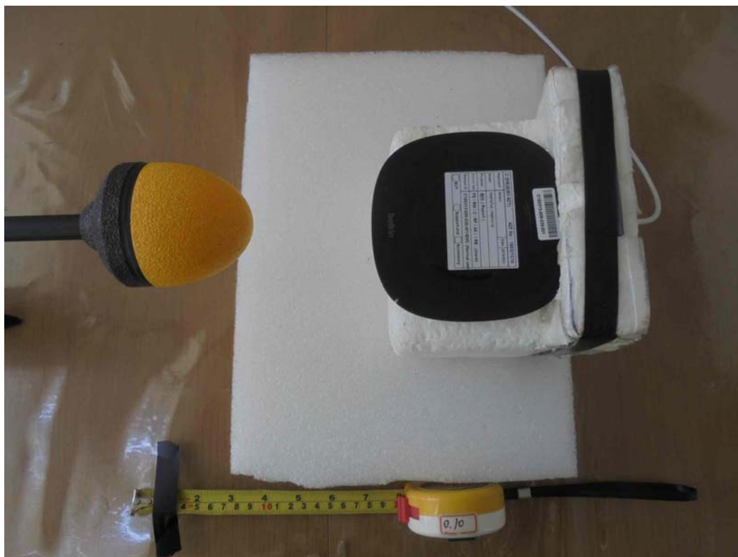
E-Field (Standby Mode - Bottom)
