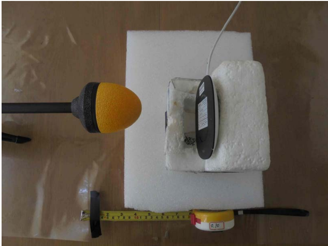
H-Field (Charging Mode with Load - Top)
