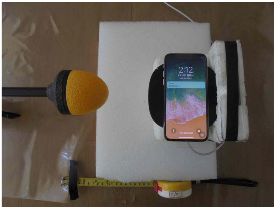
E-Field (Charging Mode with iPhone X - Z-axis)
