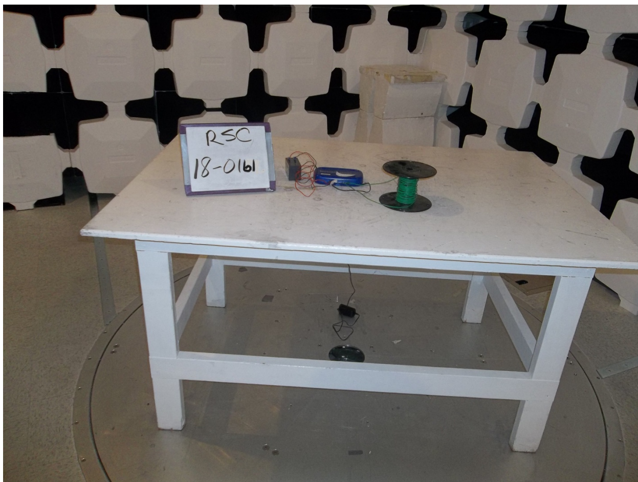
Figure 1. EUT Radiated Emissions Test Setup
