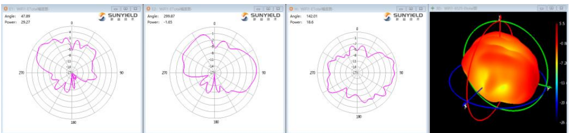
WIFI1-6525MHz 3D and 2D diagram
