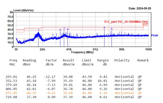
Project No.: 2407T77479E-RF Test Mode: Radar EUT Model: S532 Test distance: 3m Temp/Humi/ATM: 24.2<sup>°</sup>C/56<sup>%</sup>/100.1kPa Tested by: Zane Zhang Power Source: DC 12V from adapter
