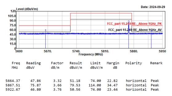
Project No.: 2407T77479E-RF Test Mode: Radar EUT Model: S532 Test distance: 3m Temp/Humi/ATM: 24.2℃/56%/100.1kPa Tested by: Wlif Wu Power Source: DC 12V from adapter
