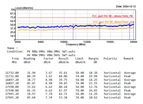
Project No.: 2407T77479E-RF Test Mode: Radar EUT Model: S532 Test distance: 3m Temp/Humi/ATM: 24.3℃/52%/100.4kPa Tested by: Wlif Wu Power Source: DC 12V from adapter
