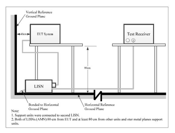
The measurement procedure of EUT setup is according with ANSI C63.10-2020. The related limit was specified in FCC Part 15.207.
