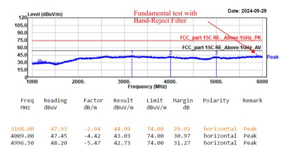
Project No.: 2407T77479E-RF Test Mode: Radar EUT Model: S532 Test distance: 3m Temp/Humi/ATM: 24.2°C/56%/100.1kPa Tested by: Wlif Wu Power Source: DC 12V from adapter
