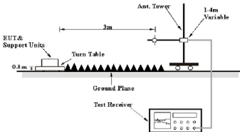
The radiated emission below 1GHz tests were performed in the 3 meters chamber test site A, above 1GHz tests were performed in the 3 meters chamber test site B, using the setup accordance with the ANSI C63.10-2013. The specification used was the FCC 15.209, and FCC 15.247 limits.
