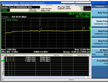
Radiated Transmitter Spurs, all modes and channels, Peak - 5GHz Wi-Fi Radio
