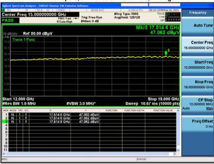
Radiated Transmitter Spurs, all modes and channels, Peak – 5GHz Auxiliary Radio
